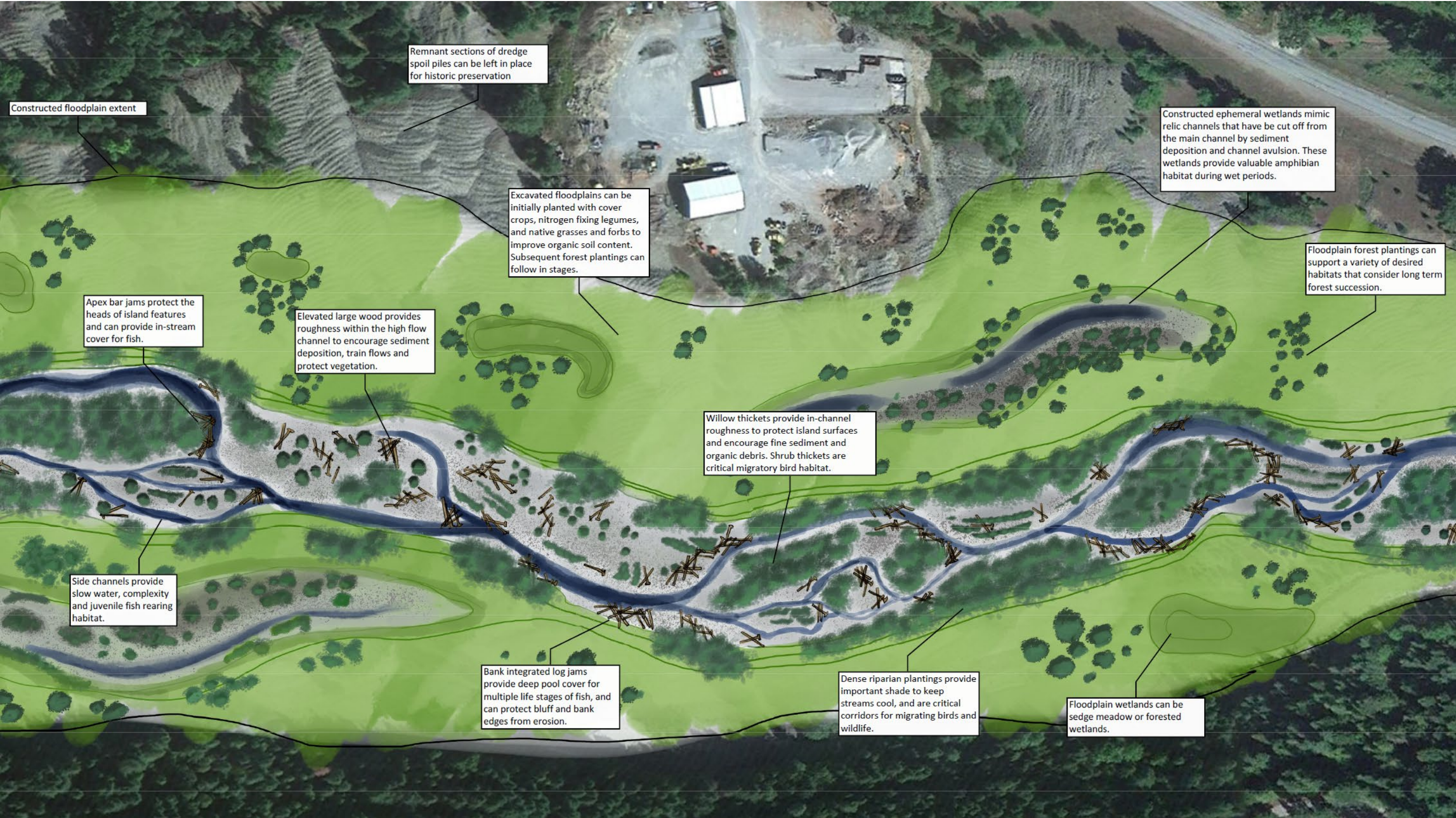
Figure 50. Illustration of proposed treatments and benefits of Alternative 2 for a section of Reach 6.
