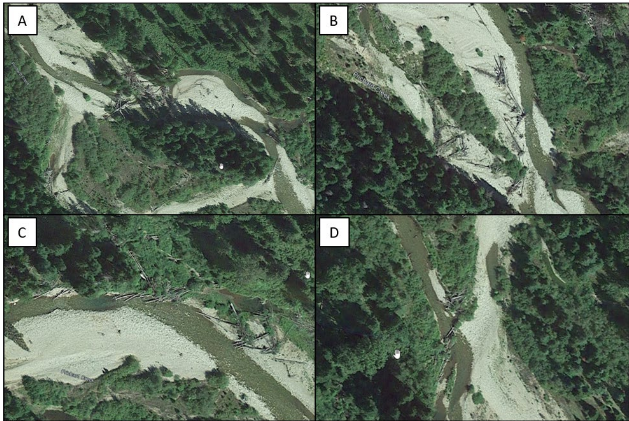
Figure 18. Large wood accumulations in lower Prichard consist mainly of a) channel spanning jams that cause channel departures or multi-threading, b) mid channel structures that guide the main channel, c) racked bank accumulations, and d) apex bar jams or racked wood at the head of vegetated islands.
